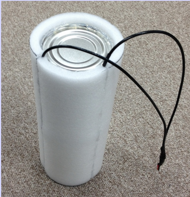
Soil moisture sensor by using cans
